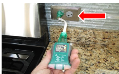
No GFCI protected/ bad wiring
