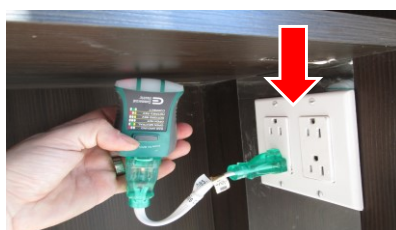
No GFCI protected/ bad wiring
