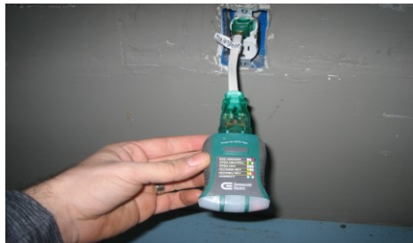
Open outlet/ no GFCI / bad ground
