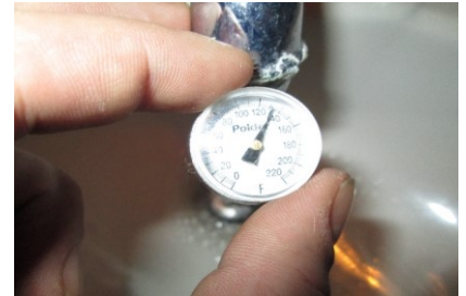
Hot water temperature is too high
